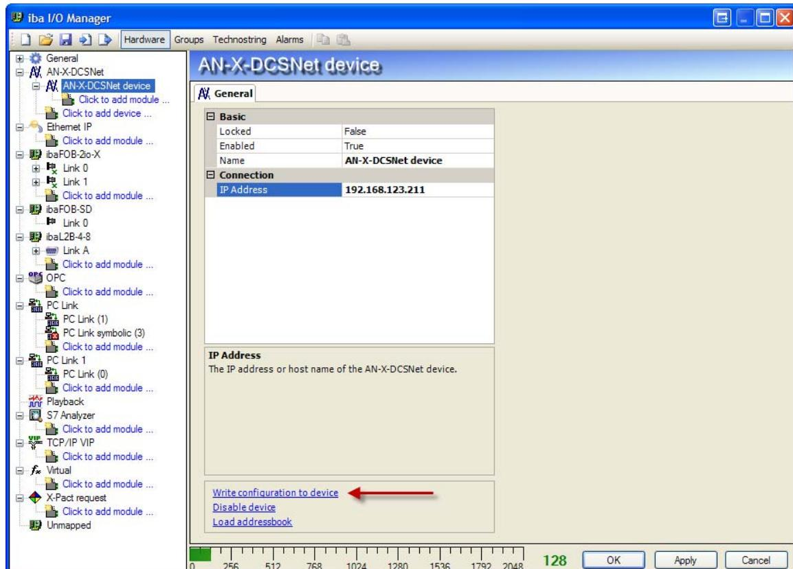
The manual write of the configuration isn't really necessary. ibaPDA will automatically write the new configuration to the device(s) when the acquisition is started.
