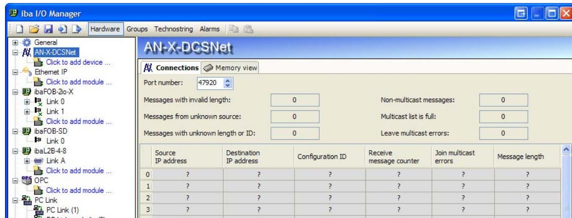
On the interface you can setup the UDP port number that ibaPDA listens to for messages from an AN-X-DCSNet device. Normally the default port number of 47920 is ok. The connections grid shows the current connections to AN-X-DCSNet devices. There are also some error counters on the interface. Check out chapter 3 for more information about these counters and the connections grid.
