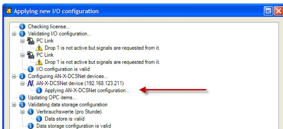
When the configuration is written to the device the device starts sending data messages to ibaPDA. You can see the actual values of the signals by going to the analog and digital tab of the AN-X-DCSNet device.
