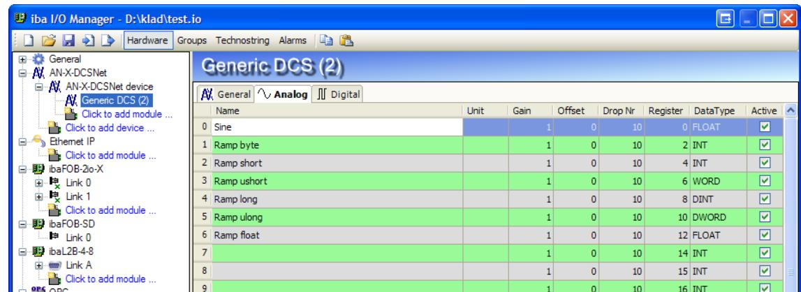
You have to specify the drop number, register number and data type for each analog signal. The supported datatypes are:
