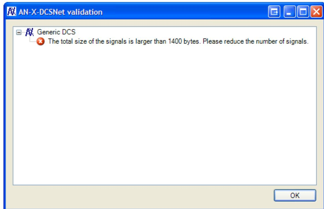
When ibaPDA creates the AN-X-DCSNet device configuration it checks if the configuration doesn't violate any of the AN-X-DCSNet limitations. If it does then the user gets an error message. These are the possible errors:
