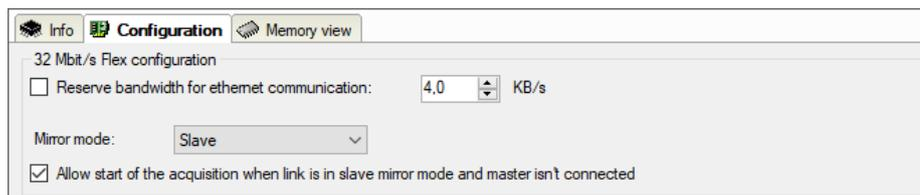
When the master ibaPDA changes the configuration while the slave ibaPDA is acquiring then the slave will automatically restart.
