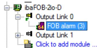
Output links without FOB alarm modules or with FOB alarm modules assigned but without any signals configured will be marked as disabled in the "Info" tab.
