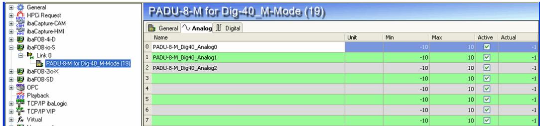
In order to display the digital signals in ibaPDA correctly, 2 modules “16 bit decoder” should be added beneath the interface “Virtual”.
