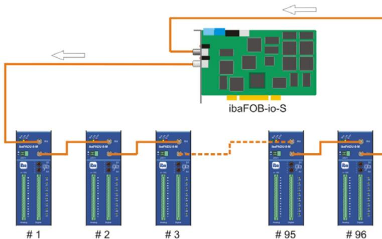
The TX port on an individual ibaFOB interface must be connected to the RX port on the first ibaPADU-8-M in the fiber-optic ring. Installed devices may be interconnected in any order (consecutive addresses are not required) provided that all devices have unique address settings. The TX port on the last device in the chain must be connected to the RX port on the respective ibaFOB interface card.
