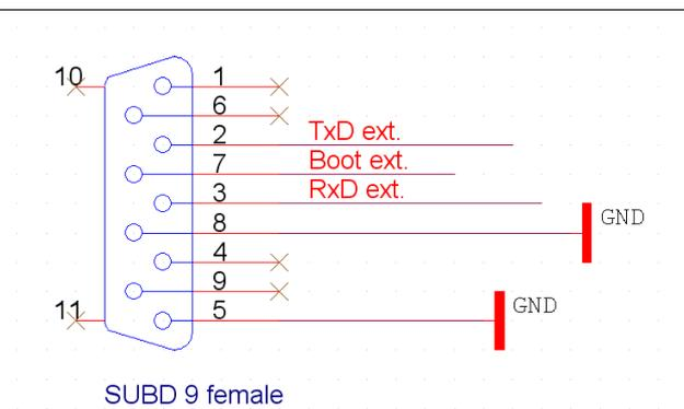
Service Interface Pinout Diagram
