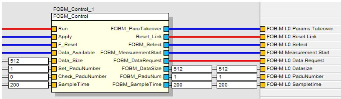
The inputs Run, Apply and F\_Reset are set by the application and control the processing, the takeover of new parameters and the resetting.
