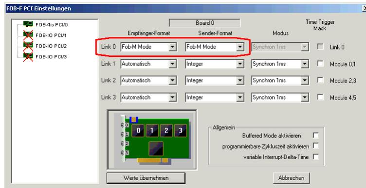
Select the corresponding ibaFOB-card in the tree on the left side. On the right side you see the settings of the selected card. Choose the line of the link which is connected to the ibaPADU-8-M and select **FOB-M Mode** in the fields for both “Receiver Format” and “Sender Format” from the pick-list. Then click on the <Apply> button.
